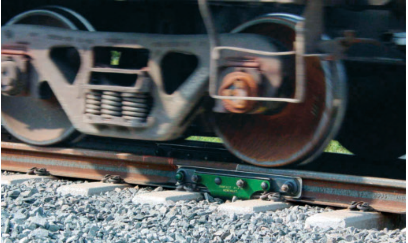
The robust NIJ-6 "Hercules" insulated joints play an essential role in current railroad circuit based signal systems by dividing the track into segments that detect train presence and activate trackside signals.
